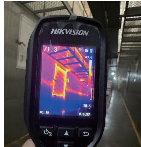
A thermal imager is used to check oven door tightness
